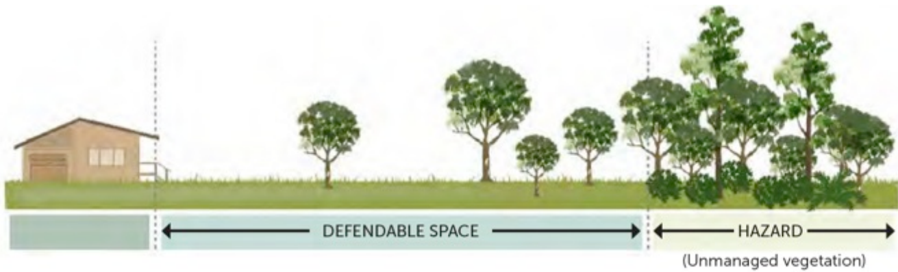
Plate 1. Defendable space around a proposed construction (Source: DTP 2026a).
