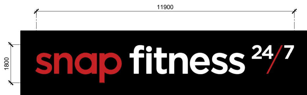
S1 - External Signage Logo fabricated from 4.5mm acrylic Depth 80-100mm illuminated opal acrylic face with black sides to block out light
