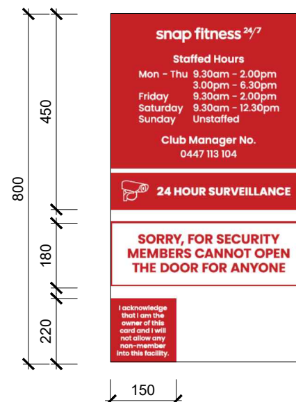
S4 - Door Signage Digital print SAV vinyl decals applied to glazing. Signage to be reverse applied (except where being applied to tinted glass).
