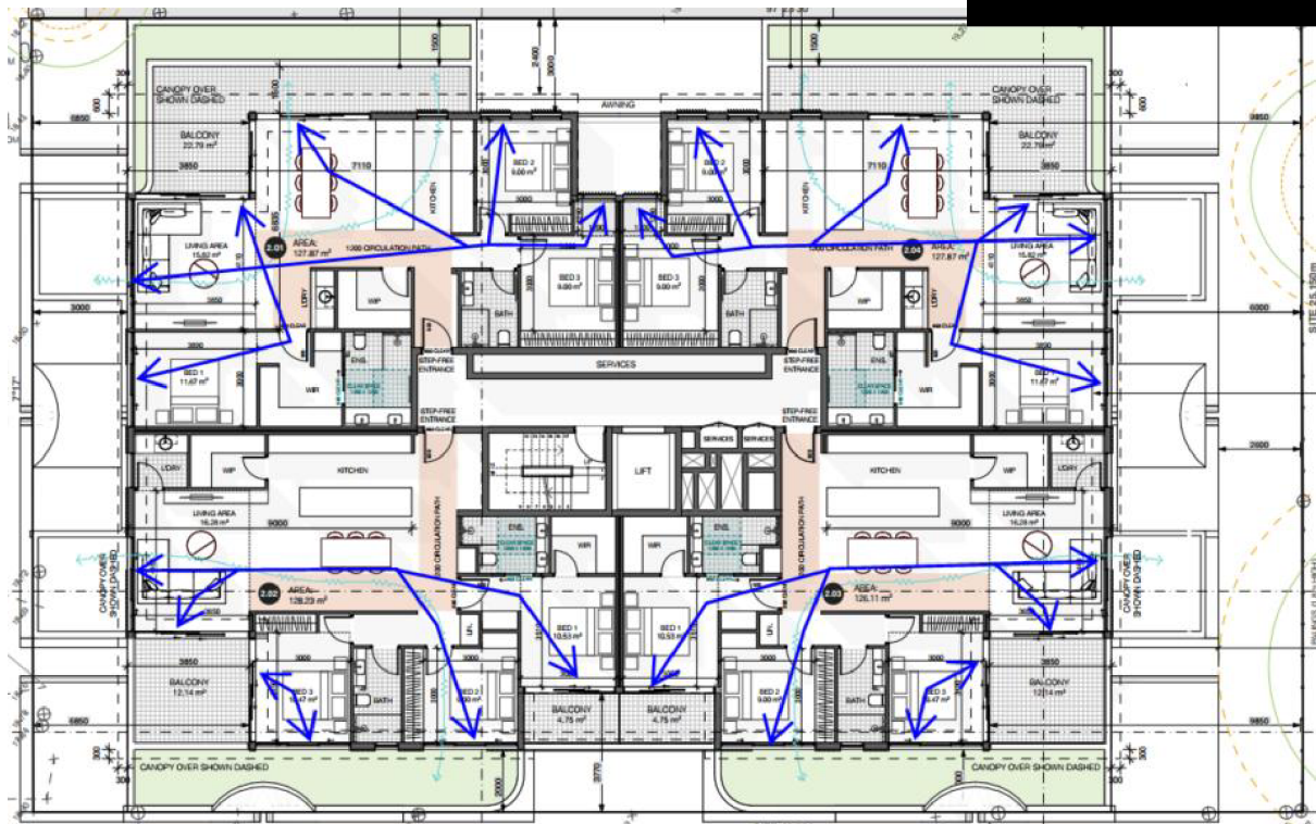
Figure 3: natural ventilation path for level 2
