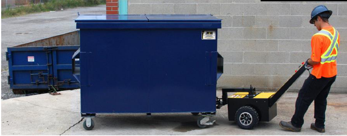
Figure 5: Example of a mechanical tug used for bin management.
