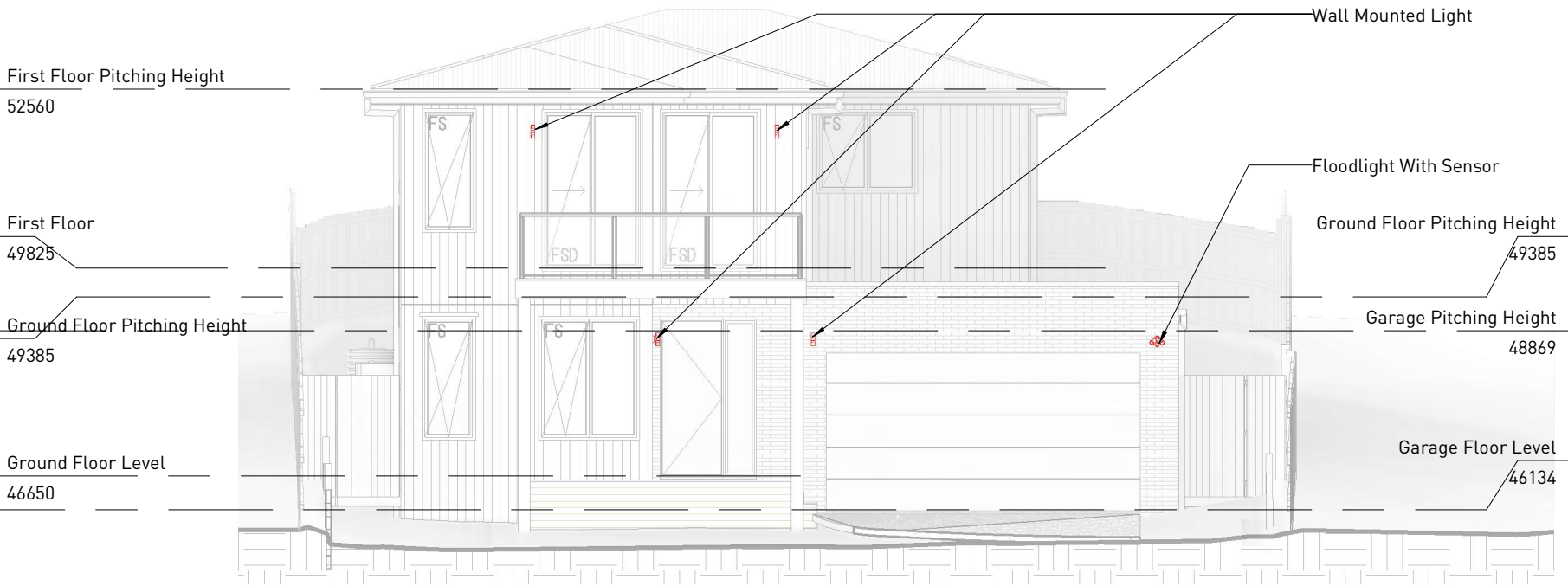
Front Elevation (Northern) Lot 2 Lighting 1 : 100
