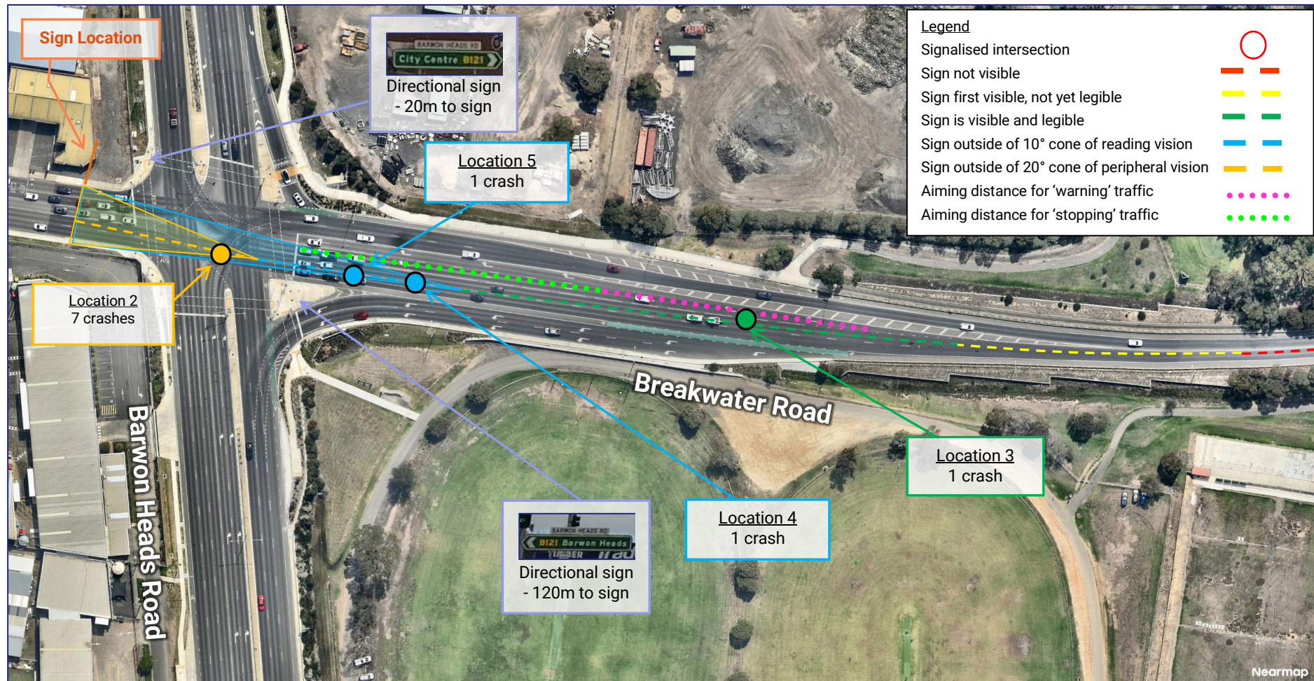
Figure B2: Crash location vs. sign visibility/legibility – Westbound approach (Source: Nearmap.com)
