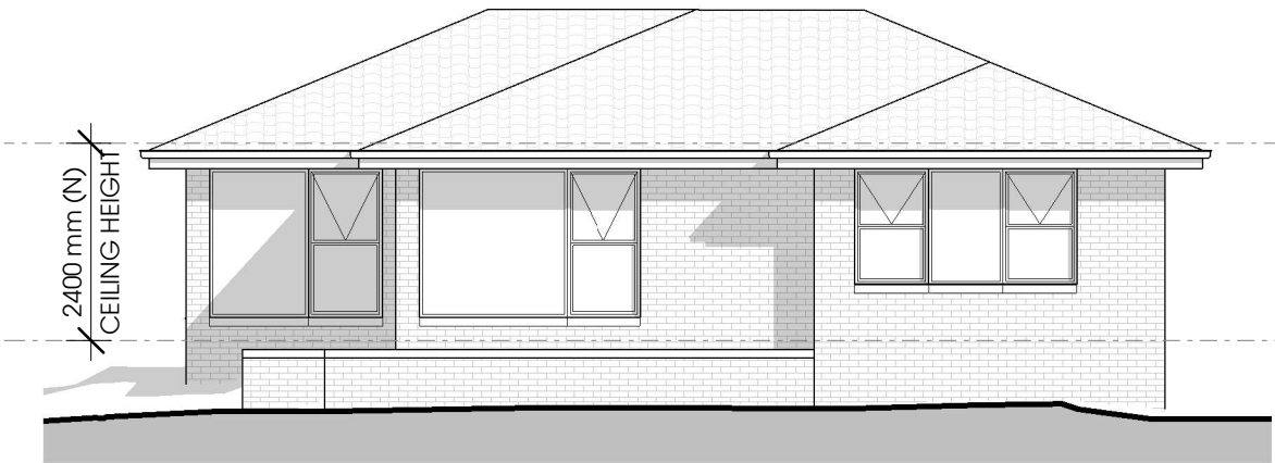
EXISTING NORTH ELEVATION
