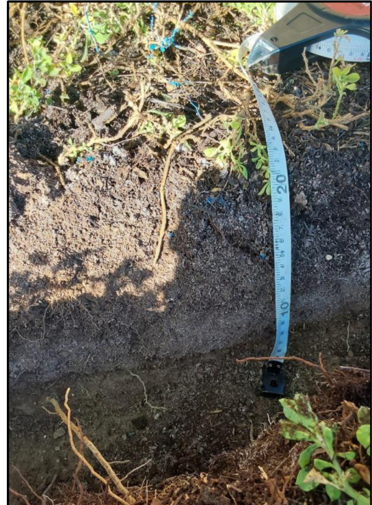
Figure 5. 130mm deep hand dug excavation.
