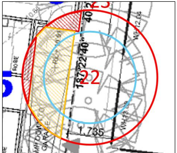
Figure 6. Tree 22 with major encroachments consisting of a large portion of shallow path construction.
