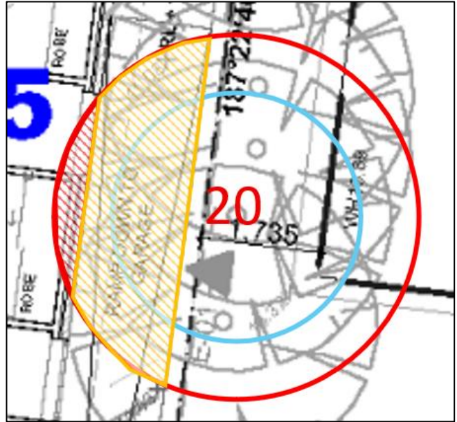
Figure 4. Tree 20 with major encroachments consisting of a large portion of shallow path construction.
