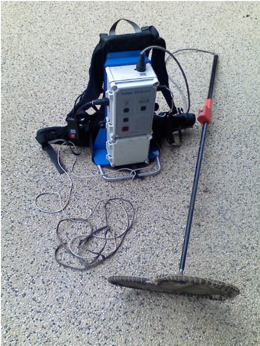
Kainga EFM 300 backpack electrofishing unit used in the surveys
