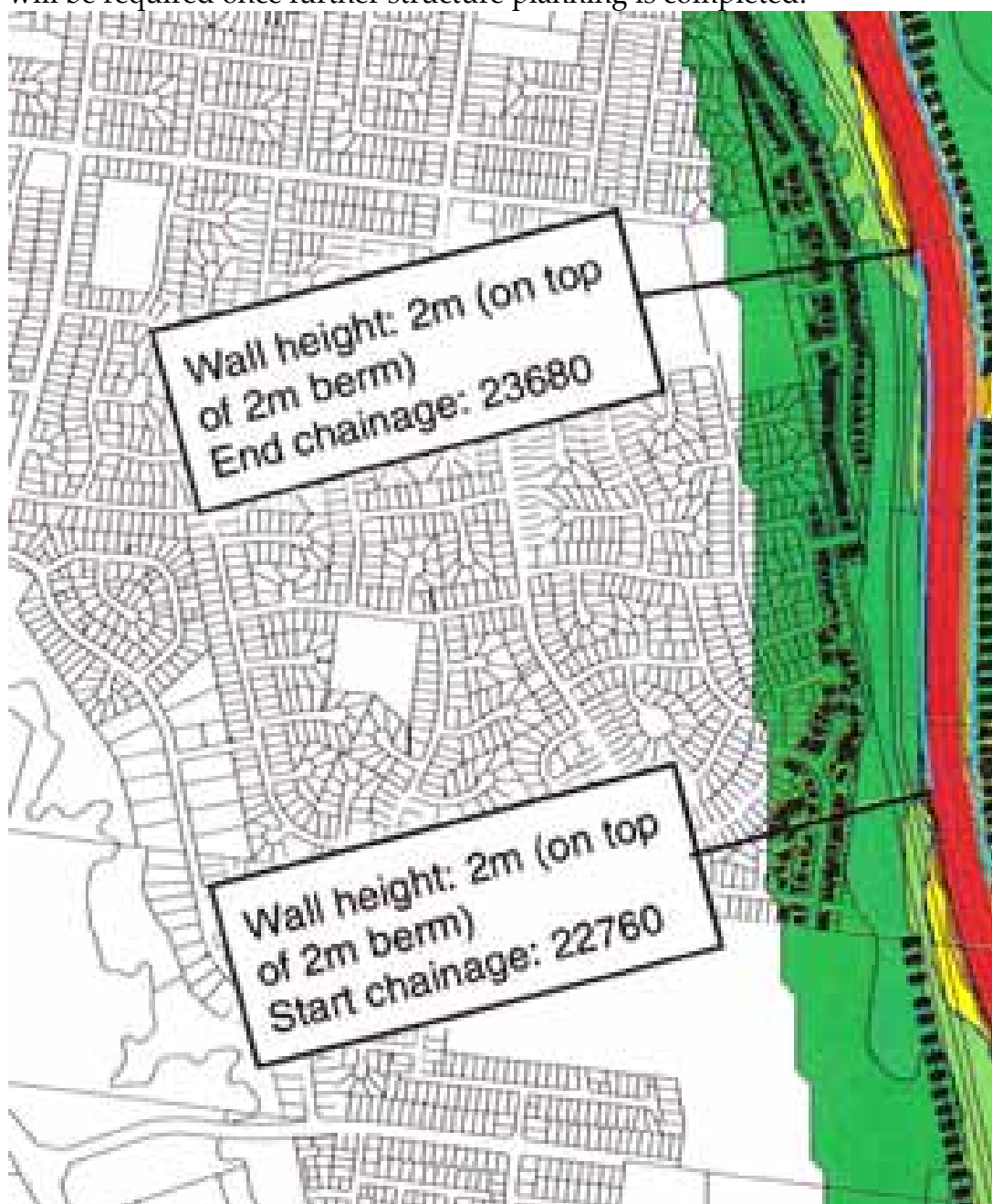
Figure 15: Northern wall location and height (on top of 2m berm – '7mm spray seal') 18
