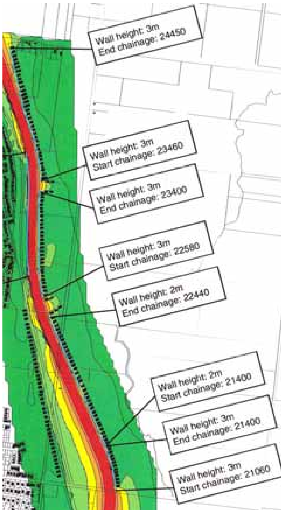
Figure 17: Indicative southern wall heights (on top of 2m berm - '7mm spray seal') 20
