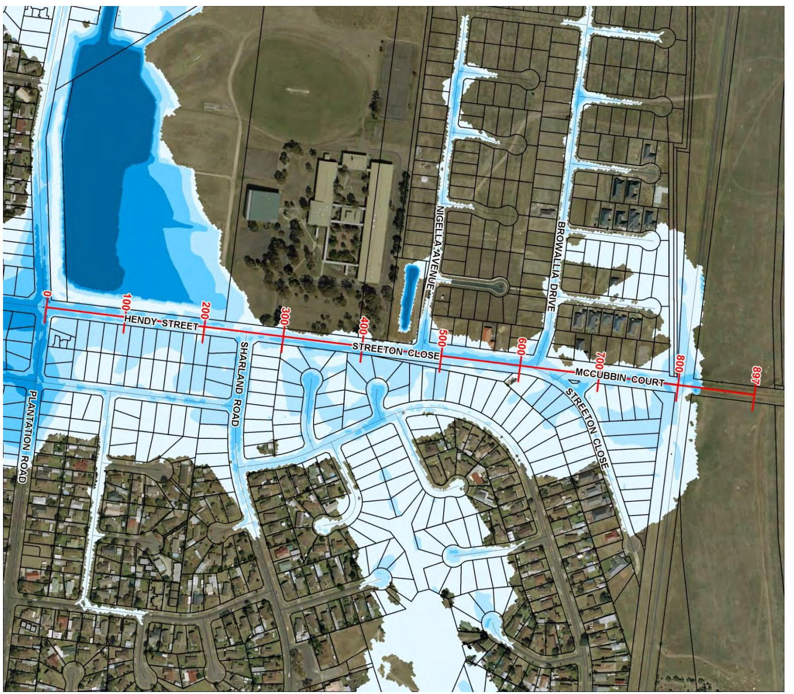
1% AEP Existing Conditions Flood Surface Longitudinal Profile Geelong Bypass to Kosciusko Avenue
