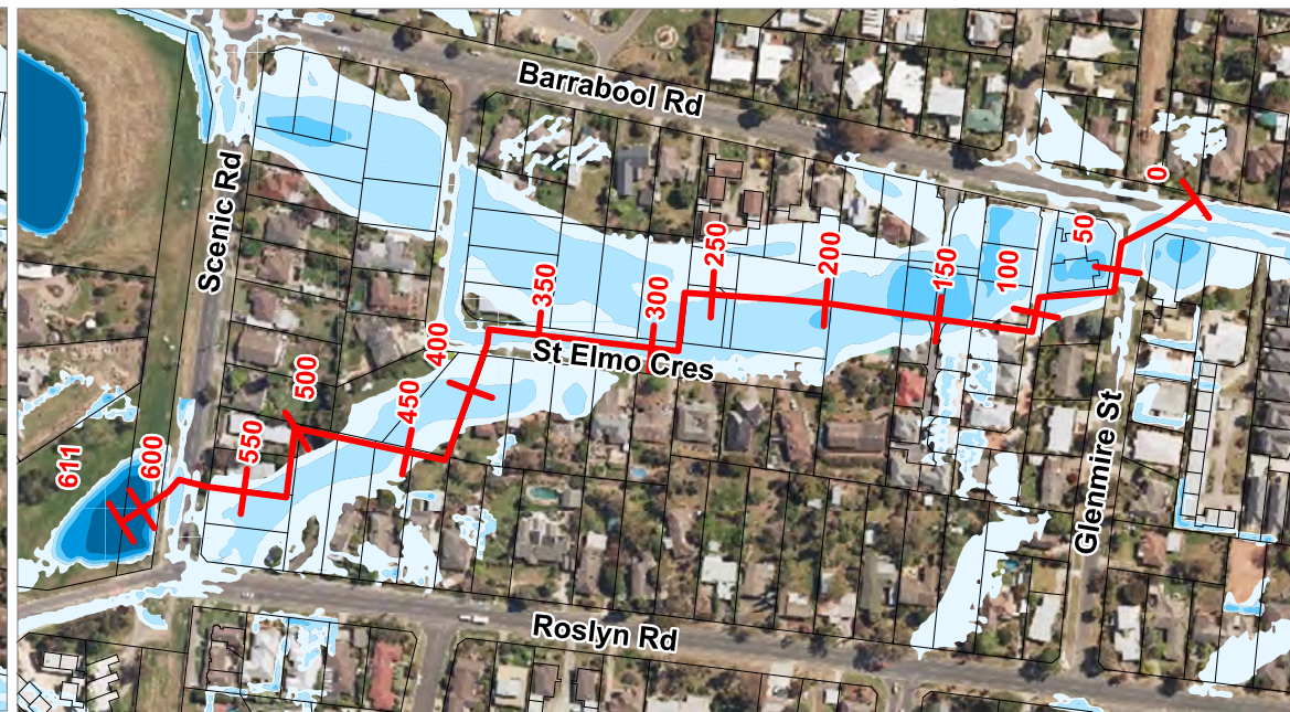
Title: 1% AEP Existing Conditions Flood Surface Longitudinal Profile Barrabool Rd Upper RB and Wandana Dr RB to Glenmire St
