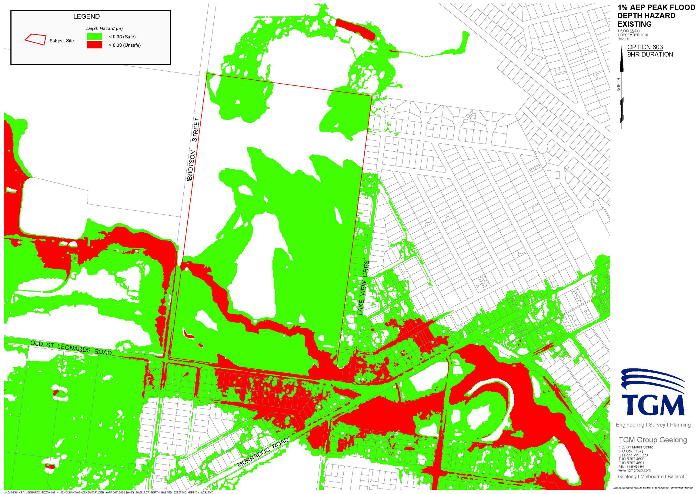
Figure 5-11 Depth Hazard Mapping – 1% AEP Existing Case
