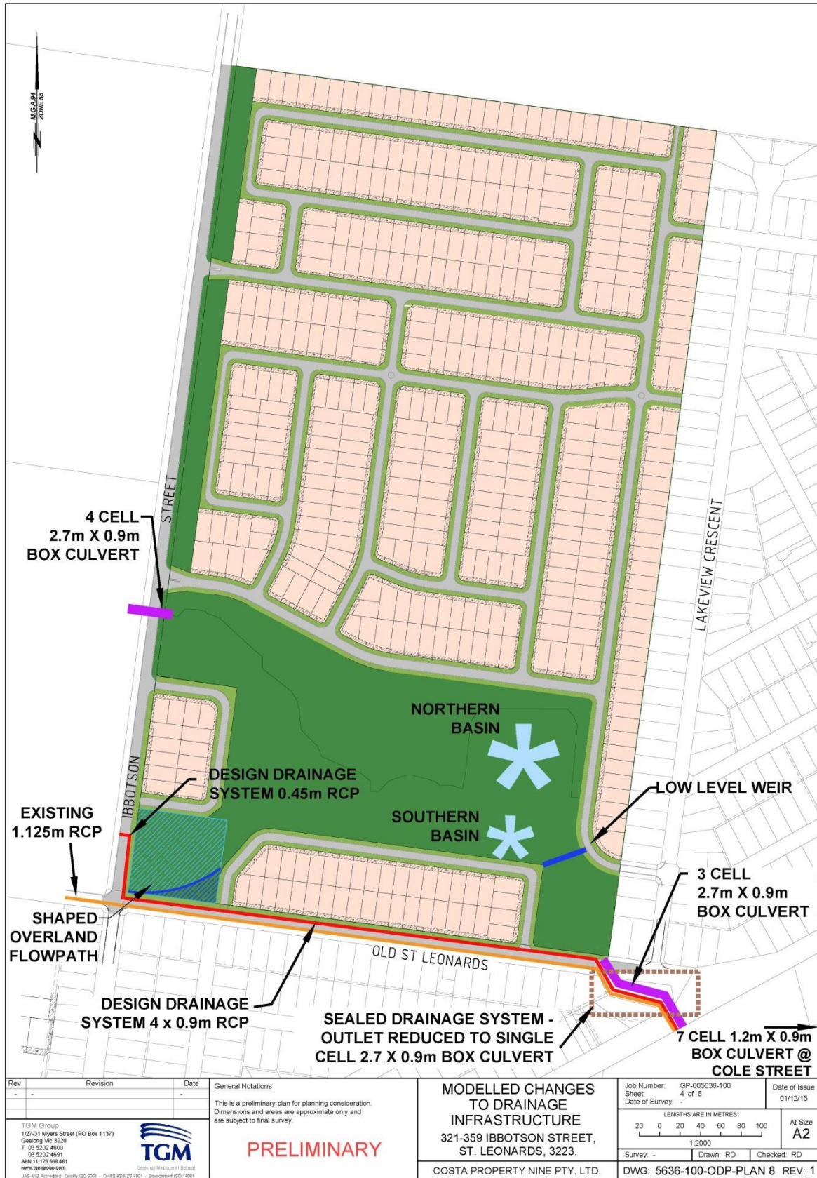
Figure 3.5: Design drainage network and infrastructure
