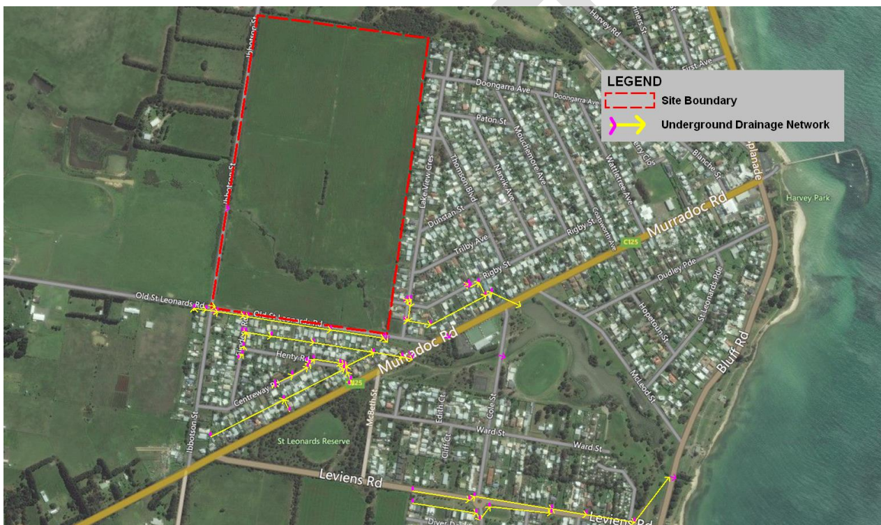
Figure 3.4: Existing underground drainage network analysed
