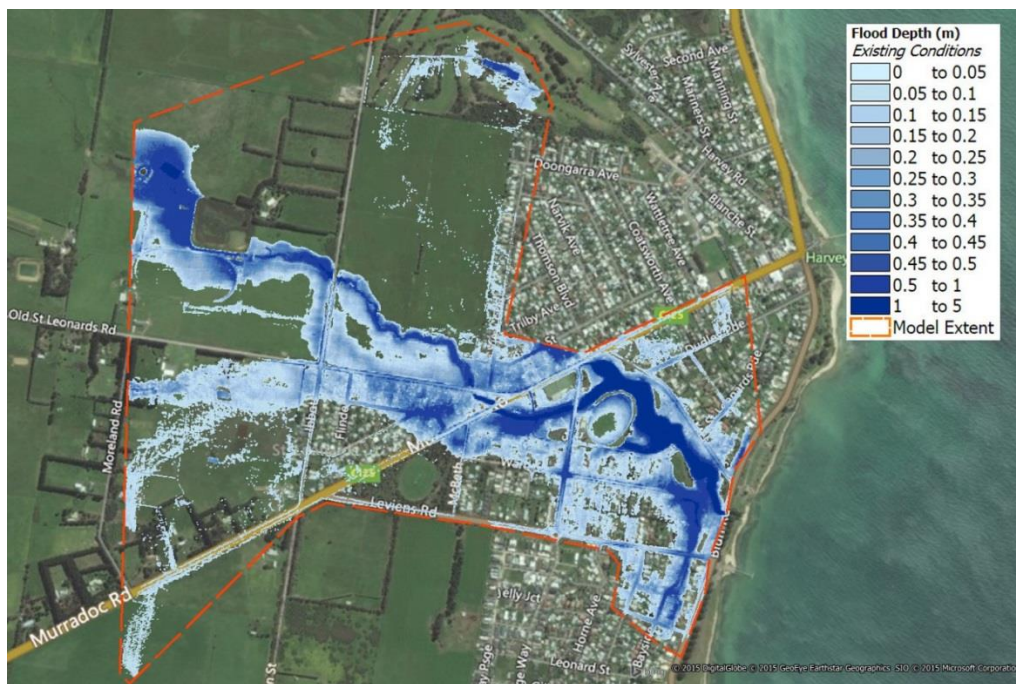
Figure 5.7: Existing 1% AEP Flood ( \geq 50 mm)
