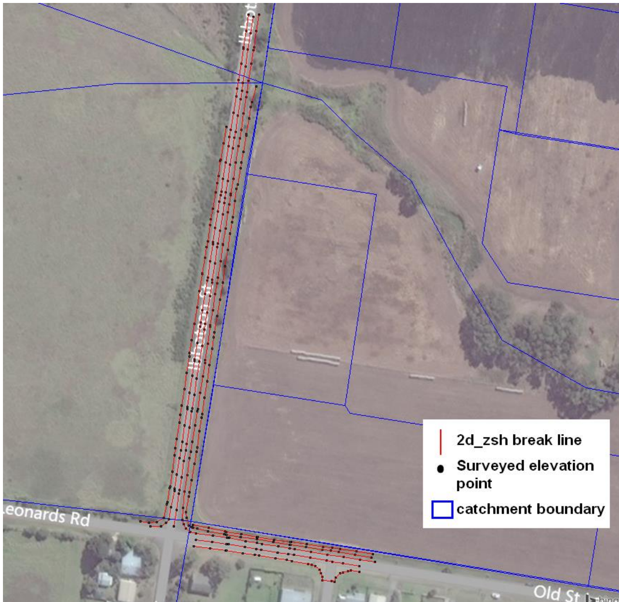
Figure 4.23: 2d_zsh break lines (Ibbotson Street & Old St Leonards Road)
