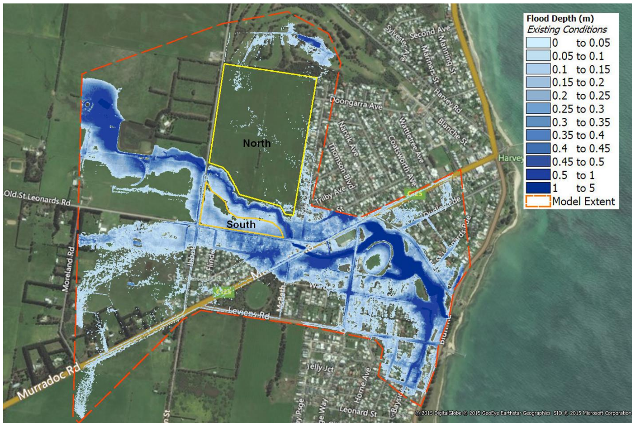
Figure A: Existing 1% AEP Flood
