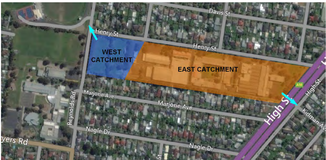
Figure 2.3: Internal sub-catchments and discharge locations
