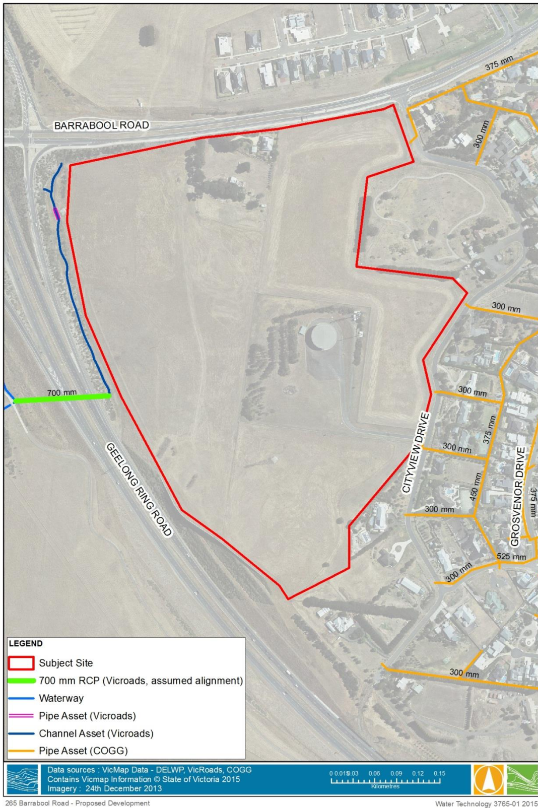
Figure 2-4 Drainage assets around the subject site
