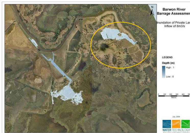
Figure 5 – Inundation of agricultural land with fixed crest height of 0.8 m and flow rate of 691 ML/day
