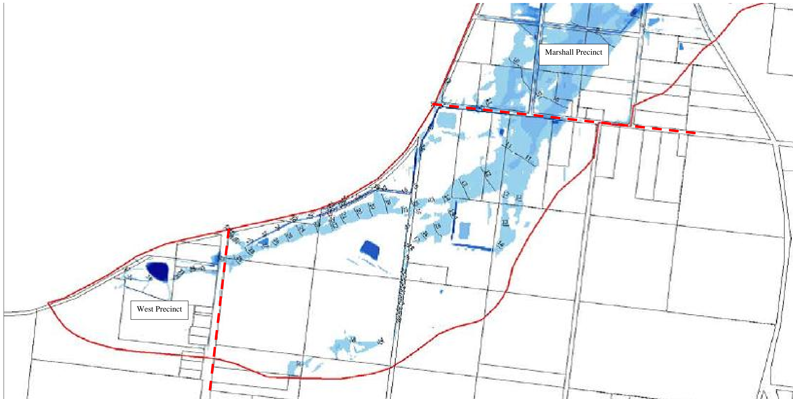
Figure 2 (Sheet 1 of 2) Armstrong Creek Horseshoe Bend Precinct (HBP) Extent and levels of inundation for 100 year ARI (existing conditions-Water Technology 2006) Reserve Road (Southeast Grovedale) Catchment
