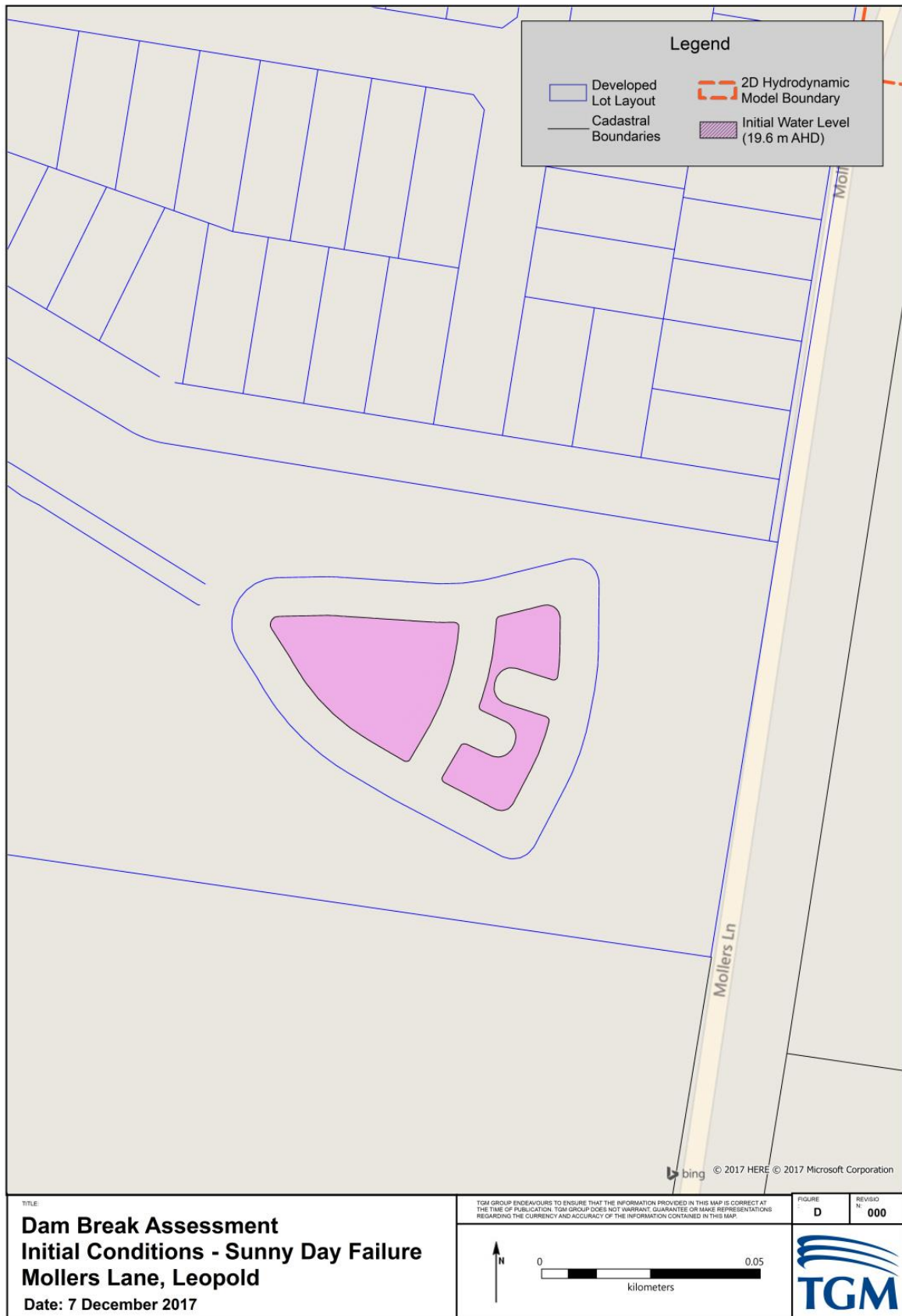
Figure 3.10: Initial Conditions - Sunny Day Failure Scenarios
