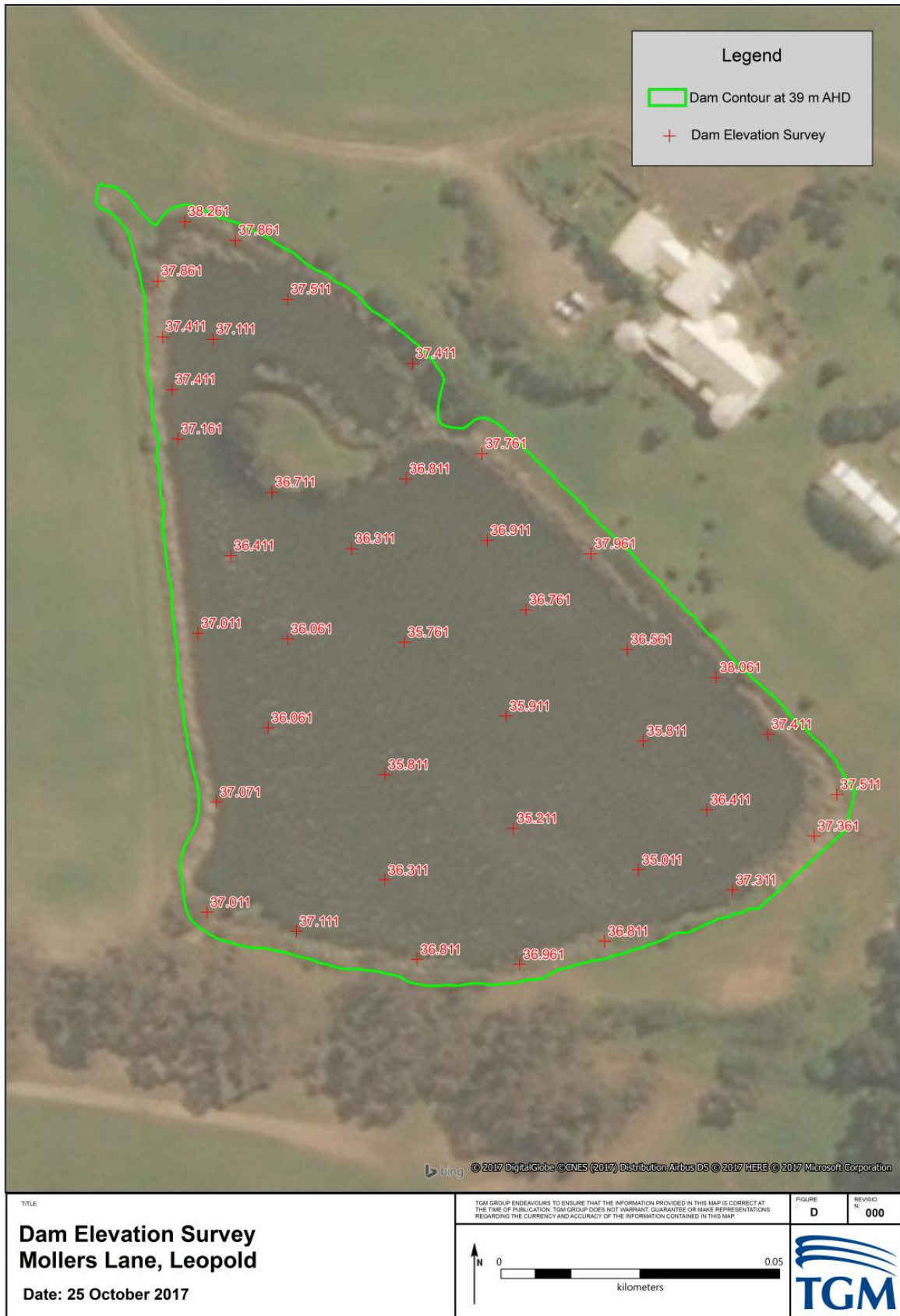
Figure 2.4: Dam Bottom Elevation Survey
