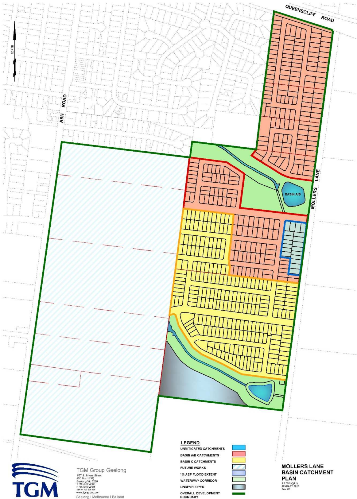
Figure 6-5: Developed site sub-catchments
