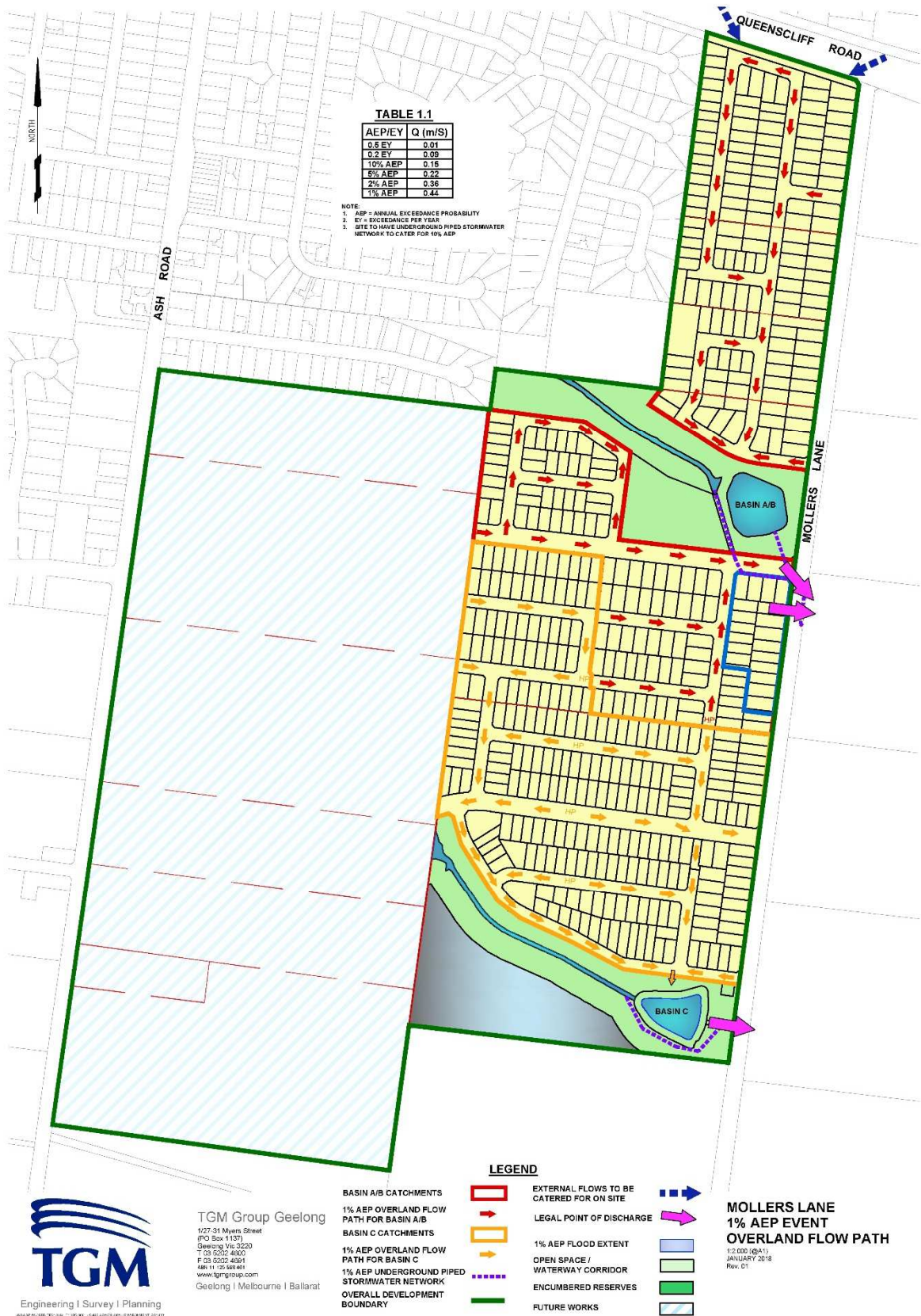
Figure 5-1: Concept Plan – Drainage Reserve Detention Basin and Wetlands
