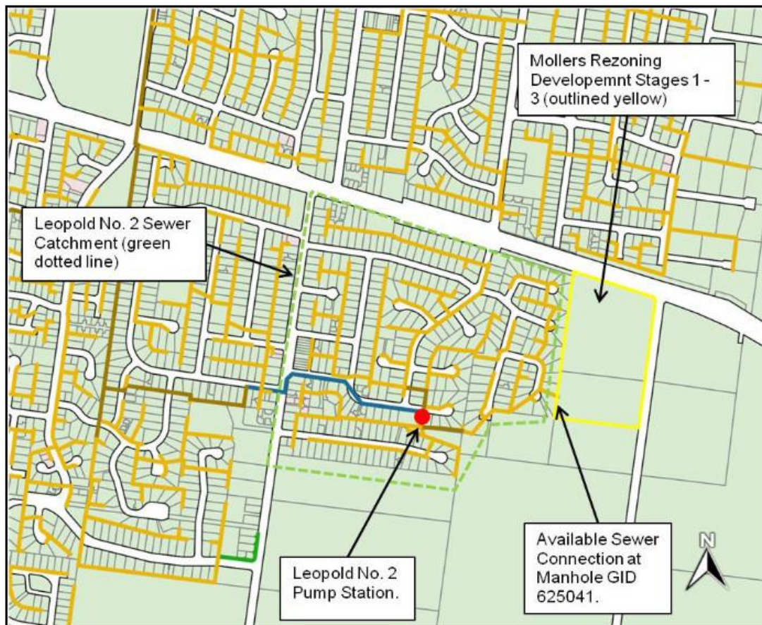
Figure 5: Sewer Connection for Stages 1, 2 & 3 5
