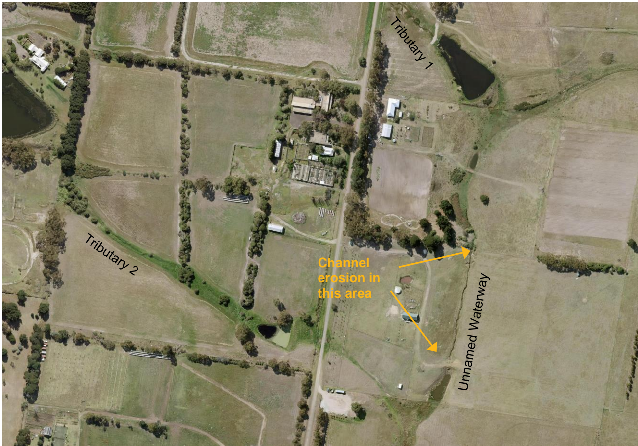
Figure 6-6 Aerial Image April 2021, evidence of erosion in Unnamed Waterway (Source: MetroMap)
