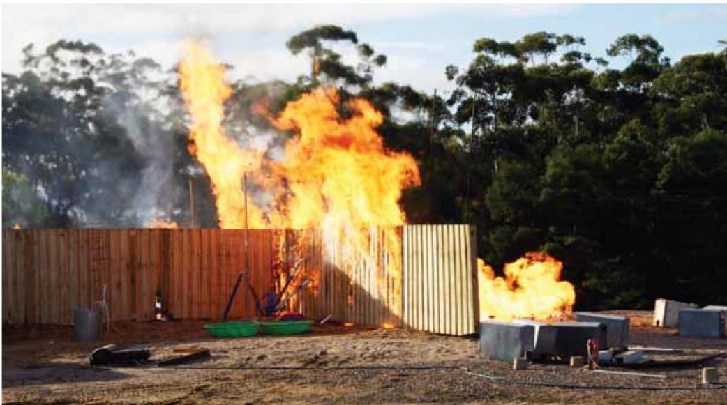
◀ Testing of different types of fencing was conducted at the NSW Rural Fire Service Experimental Testing Site at Mogo on the south coast of NSW in 2005.
