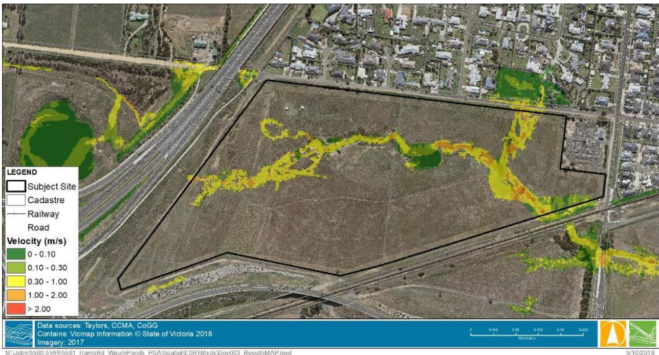
FIGURE 5-2 1% AEP FILTERED MAXIMUM VELOCITY – EXISTING CONDITIONS
