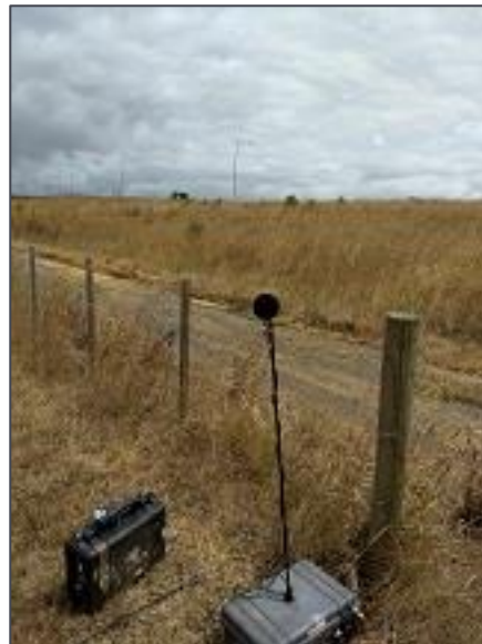
Figure 5: Unattended noise monitor – Location 2
