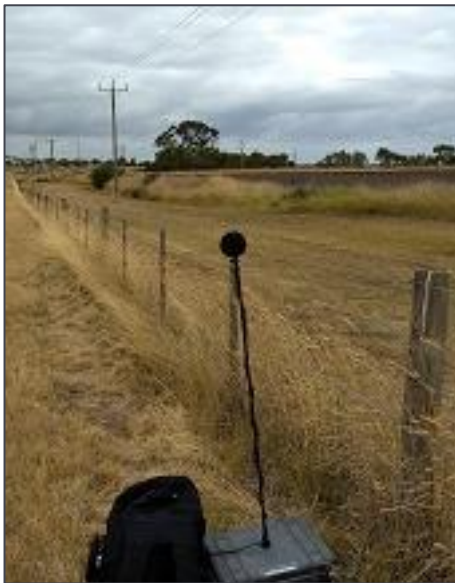
Figure 8: Unattended noise monitor – Location 5
