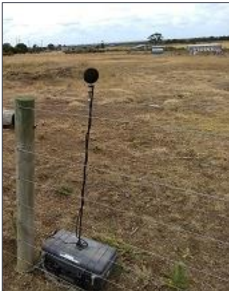
Figure 4: Unattended noise monitor – Location 1
