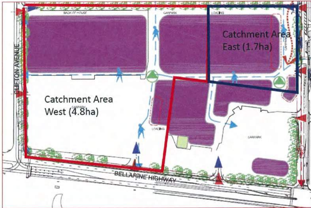
Figure 2: Sub-catchment Areas and Existing Drainage System
