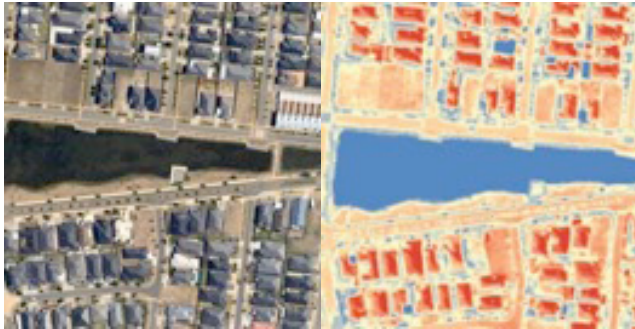
COOLING EFFECTS OF WATER WITHIN THE URBAN LANDSCAPE, BOTH THROUGH EVAPORATIVE COOLING AND PROVIDING THERMAL MASS (IMAGE: AECOM AND MONASH UNIVERSITY)
