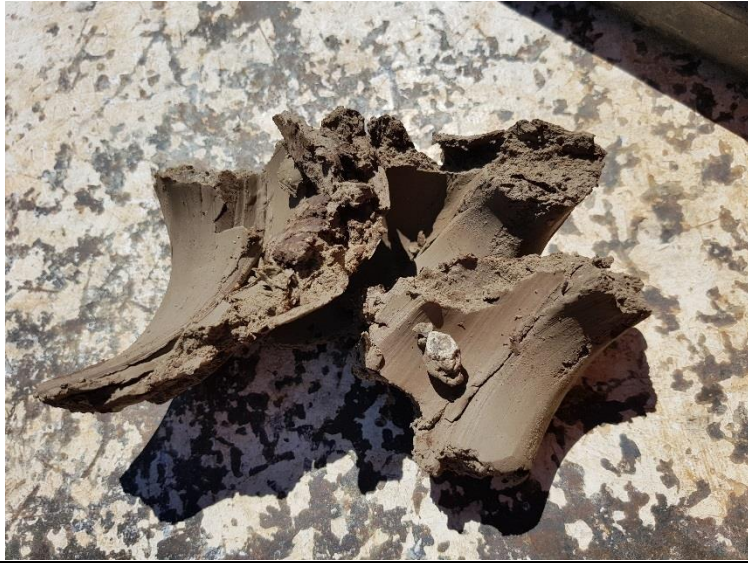
Clay (CH), highly reactive, brown, dry to damp, stiff (borehole 14, 0.5m-0.6m )
