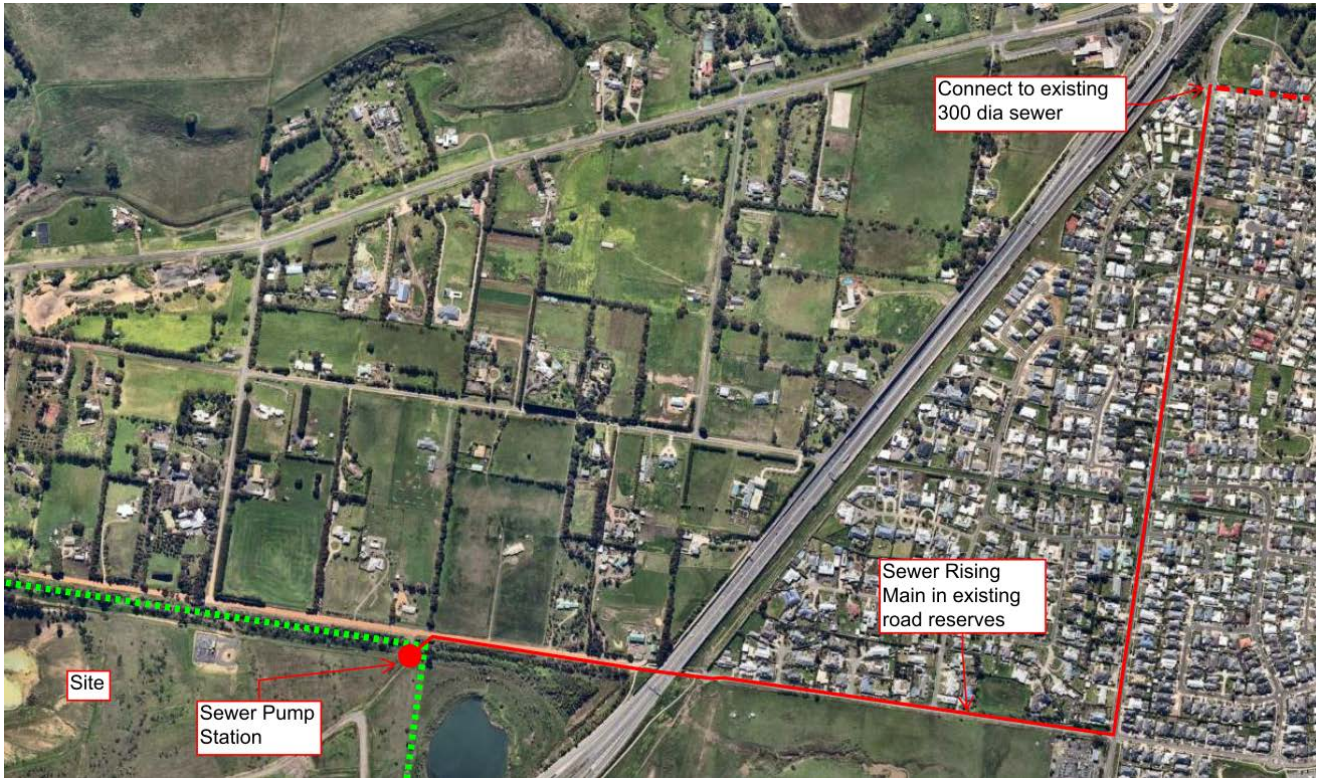
Figure 5-2 Sewerage Strategy – Initial Development
