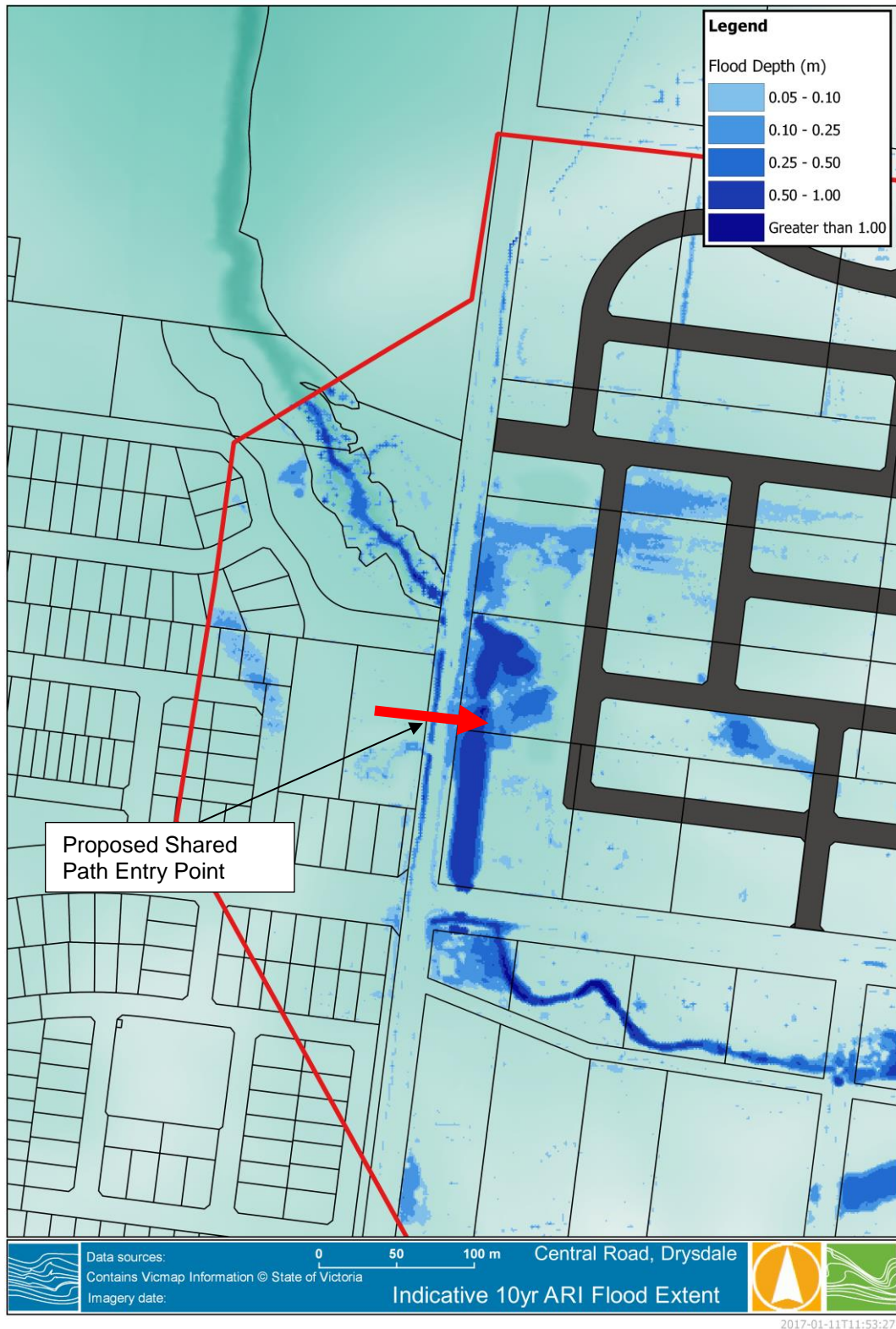
Figure 6-11 – Indicative 10% AEP Flood Extent (9 hour duration)
