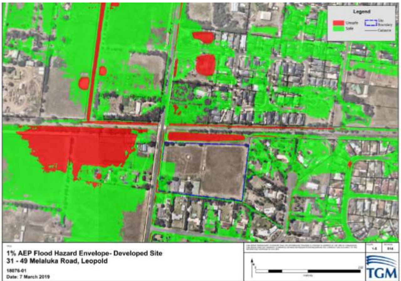
Figure 8 1 percent AEP Hazard Envelope at Developed conditions
