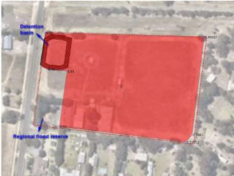
Figure 6 Filled area and basin location 10
