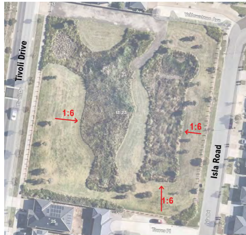
Figure 4.38 - Aerial photo of Sapphire Reserve with batter slopes
