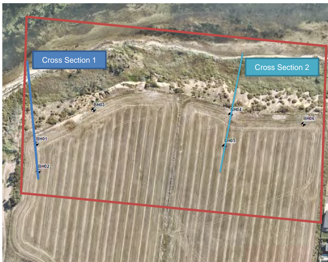
Figure 8-1: Excerpt from Nearmap (Dec 2022) depicting Extent of the of Current investigation, Approximate Borehole Location and Cross Section Locations
