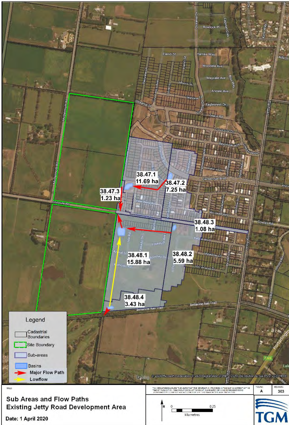
Figure 3.3: Jetty Road Development Catchment Plan
