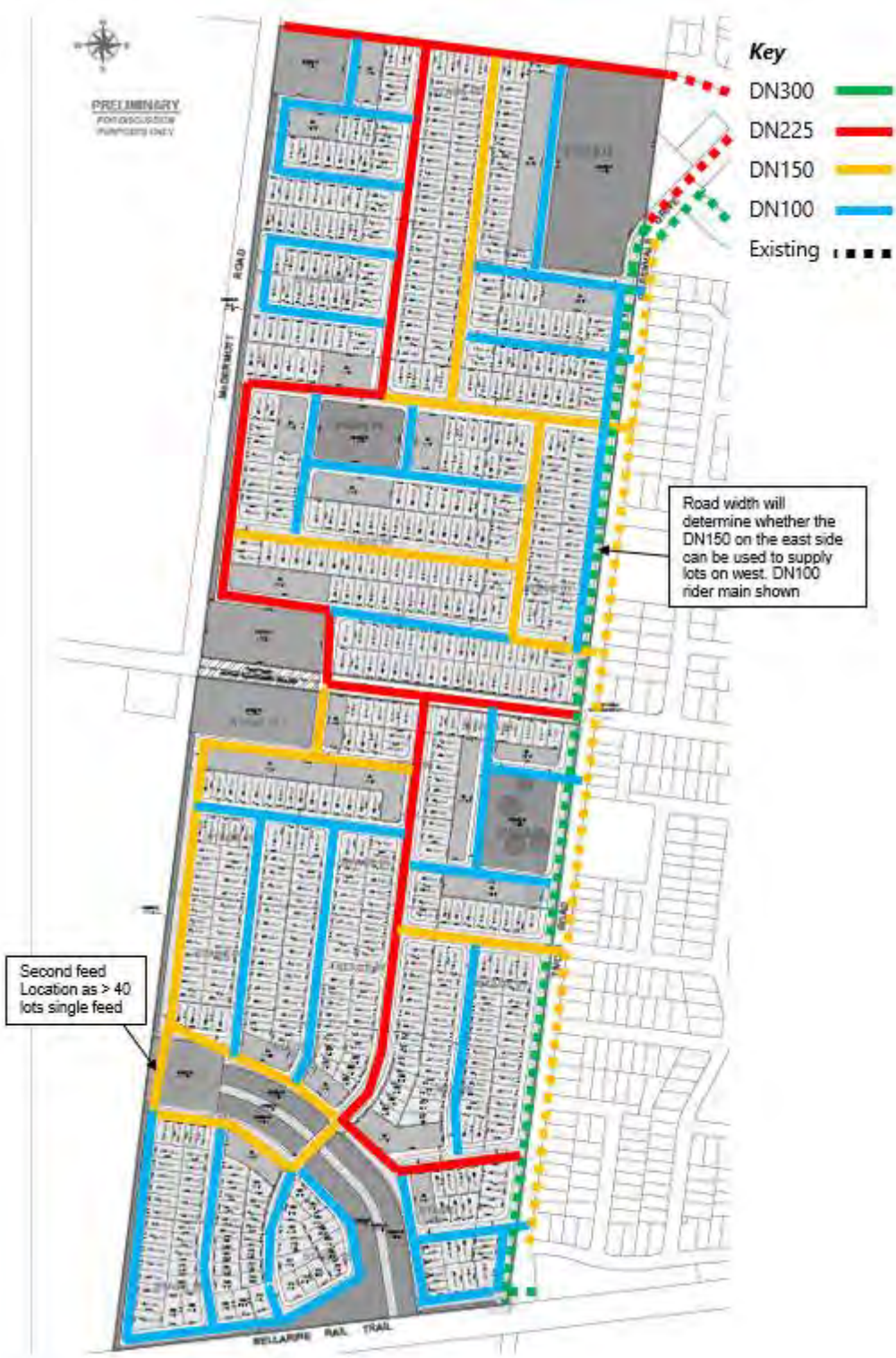
Figure 1 – Water main alignment
