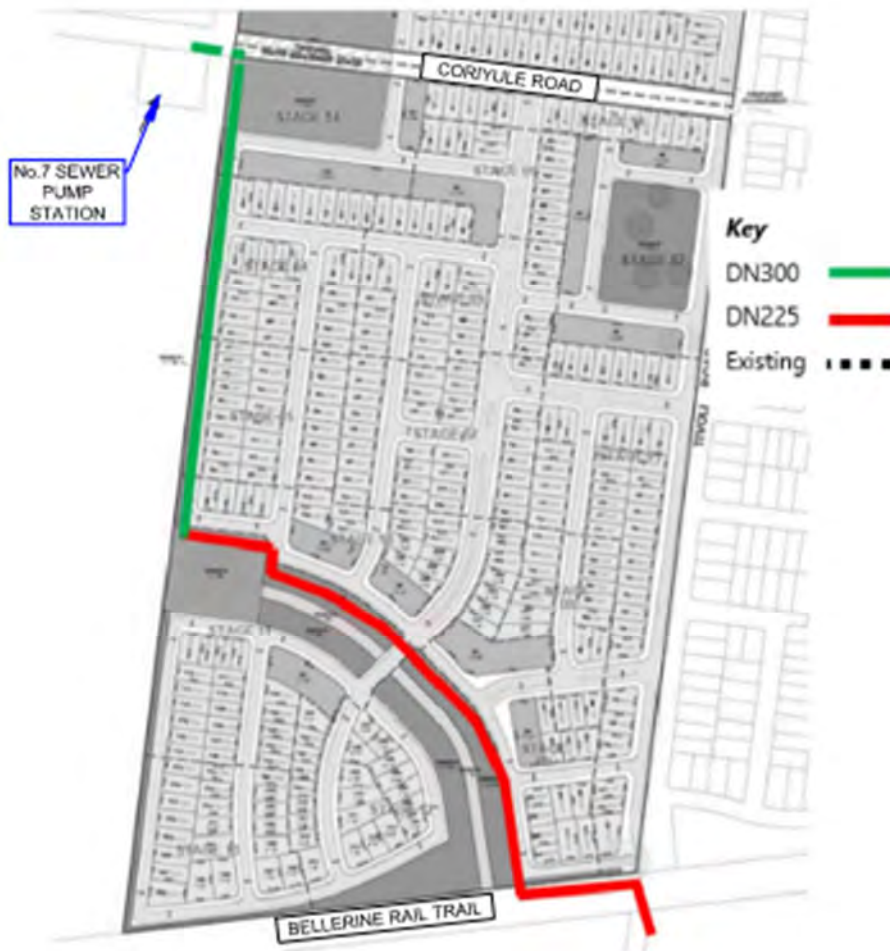
Figure 3-3 Trunk sewer horizontal alignment
