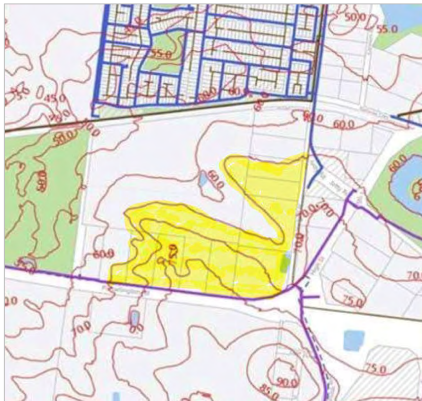
Figure 10: Land above 65 m AHD – proposed to be connected to ex. main in Portarlington Rd (Purple Line)
