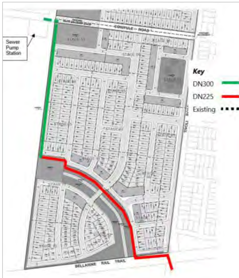
Figure 6: Outfall Sewer Alignment – Proposed sizing
