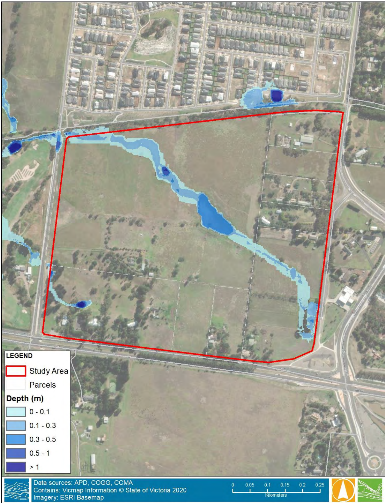
FIGURE 3-6 10% AEP FLOOD DEPTH – EXISTING CONDITIONS
