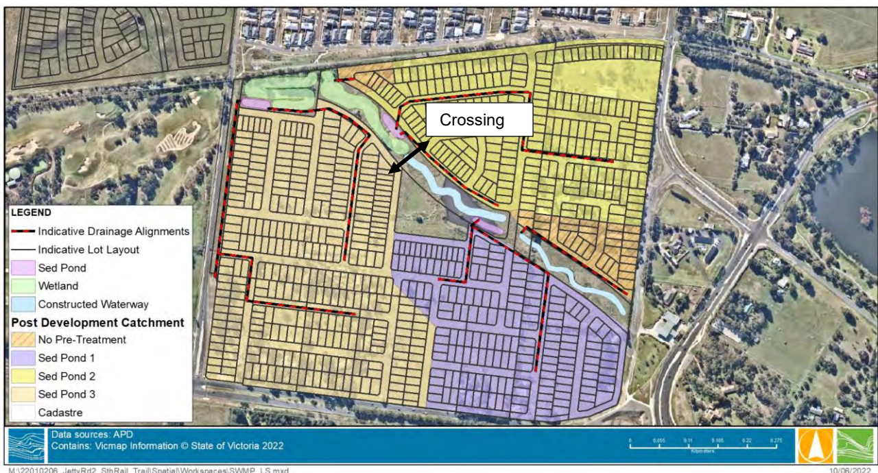
FIGURE 6-6 POTENTIAL WATERWAY CROSSINGS
