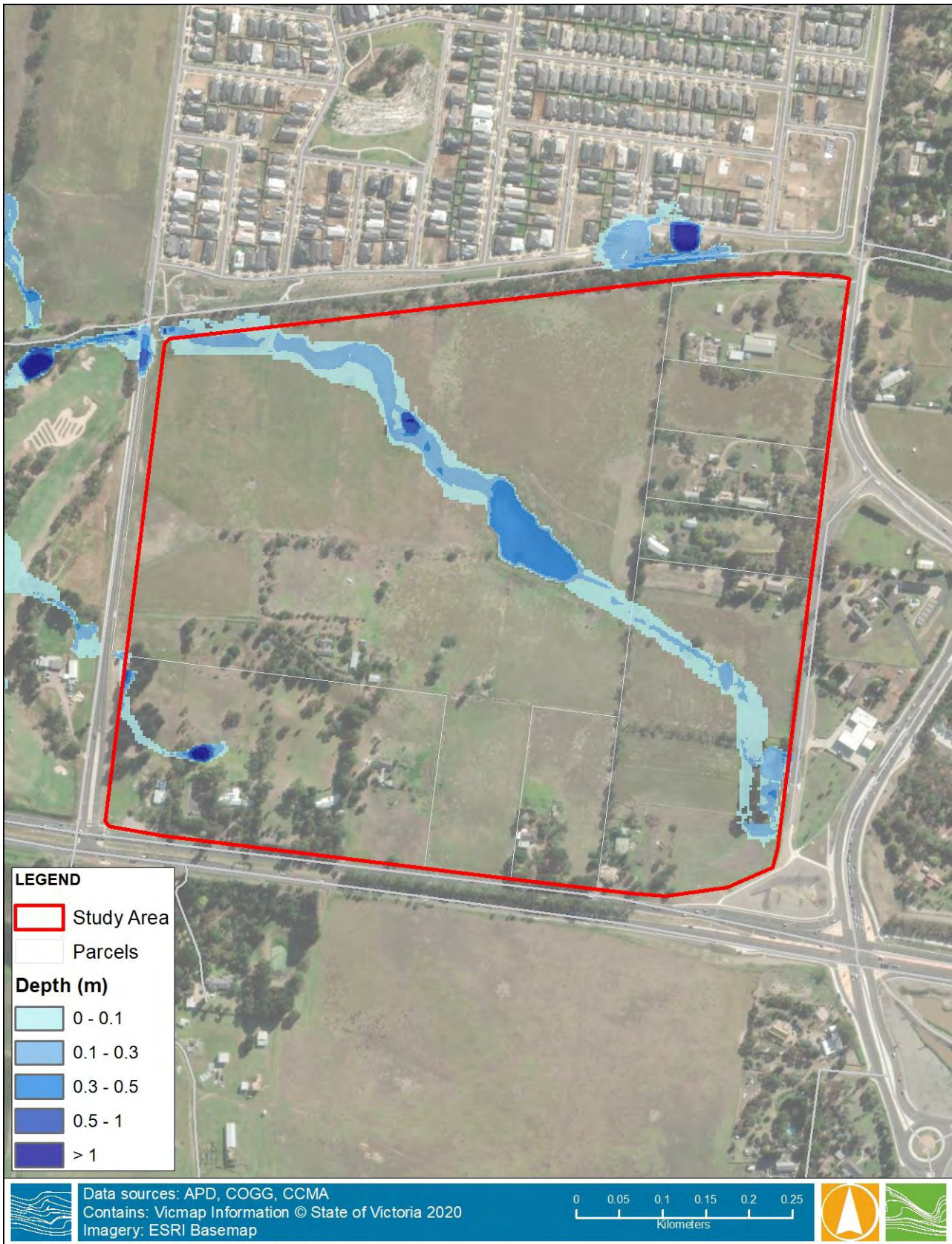
FIGURE 3-6 10% AEP FLOOD DEPTH – EXISTING CONDITIONS
