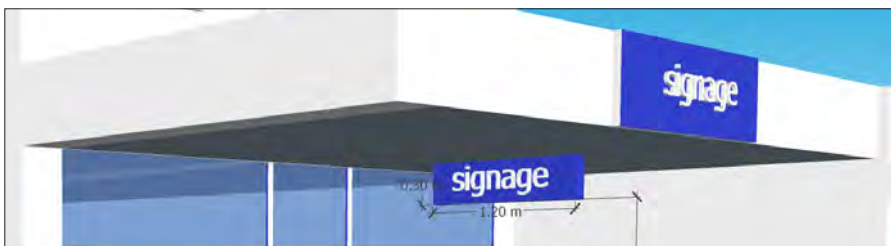
Figure 2: Under-verandah sign clearance
