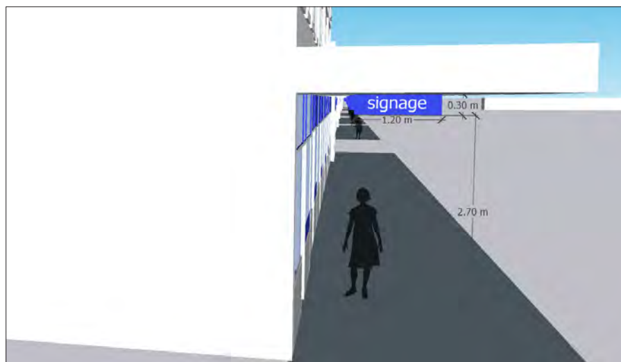
Figure 4: Under-verandah sign at right angle to building
