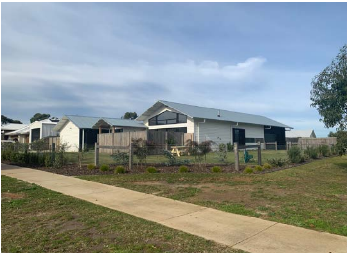
Example corner site with post and wire front fence and timber paling
