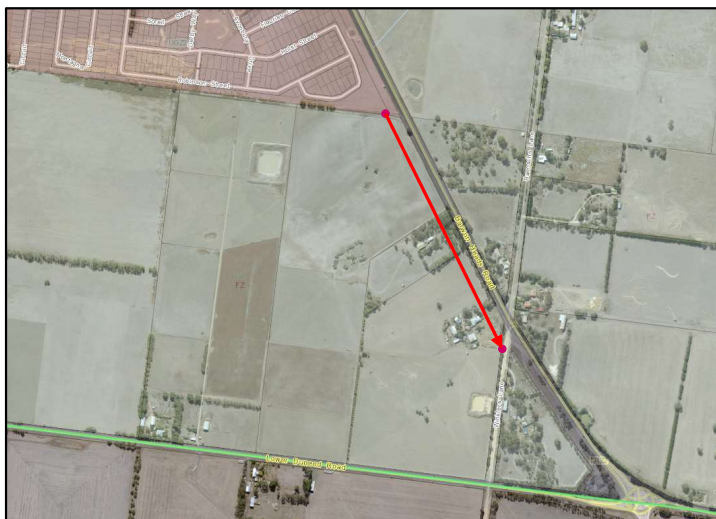
Figure 35 – Missing road widening reservation between the UGZ and Winklers Lane (red line). Source: CoGG.
