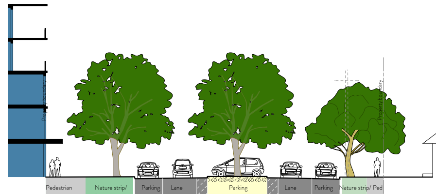
Figure 126. Lonsdale Street (East), proposed typical cross section
