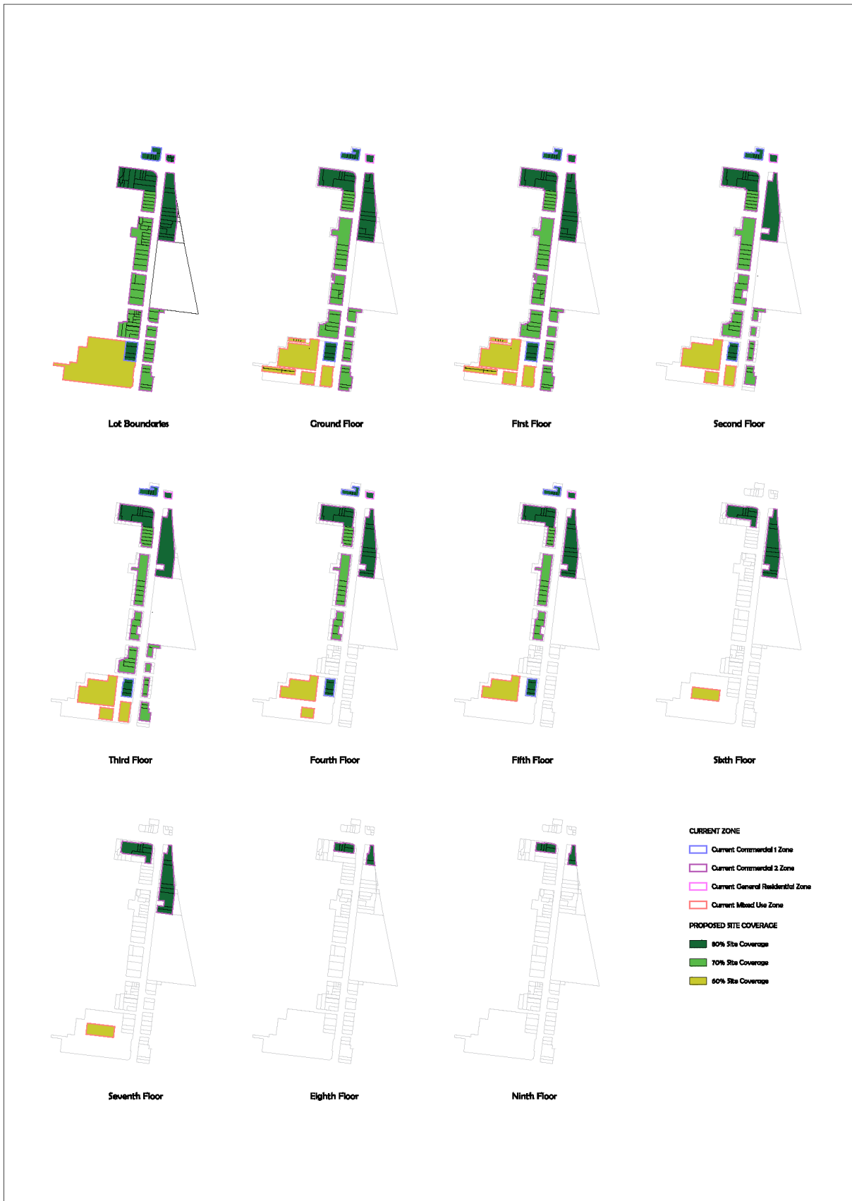
Figure 2 Horizontal sections of the 3D model at each floor - by current zone and proposed site coverage
