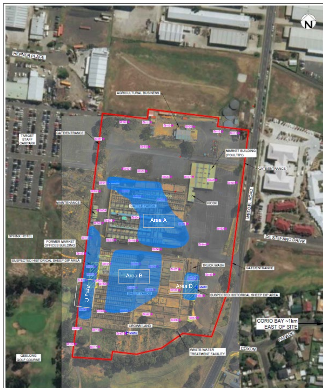
Figure 3-3: Soil contamination areas of concern identified in 2018 ESA (Source: Coffey (2018))
