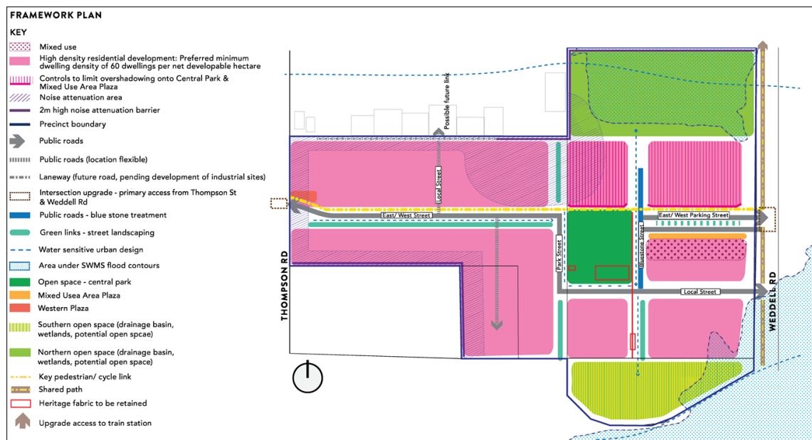
Image 2: Plan 1 - Future Urban Structure in proposed Comprehensive Development Plan. Residential land is coloured in pink and central park in dark green.
