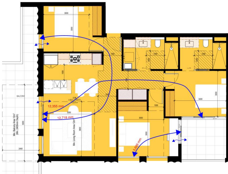
Figure 7: Natural Ventilation 3 Bed Apartment
