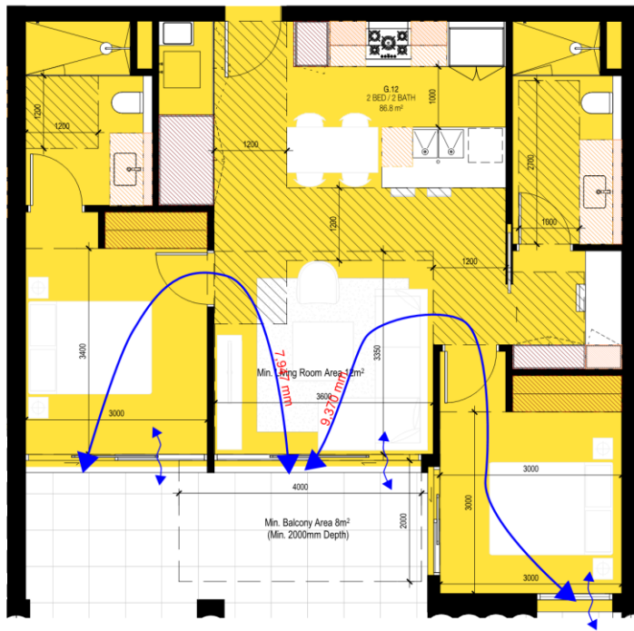
Figure 6: Natural Ventilation 2 Bed Apartment
