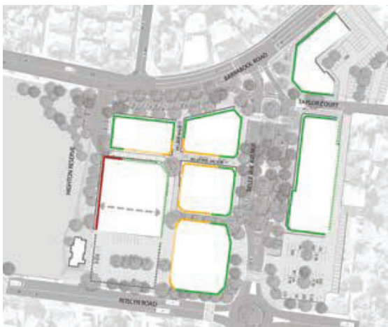
Figure 31. Street wall, building heights and setbacks plan
