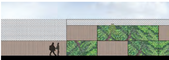
Figure 21. Green Wall Elevation C-C
