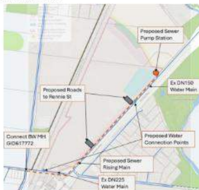
Figure 1 - Recommended Water and Sewer connections
